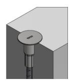
Mount the cap in the socket after removing the nailing plate.
